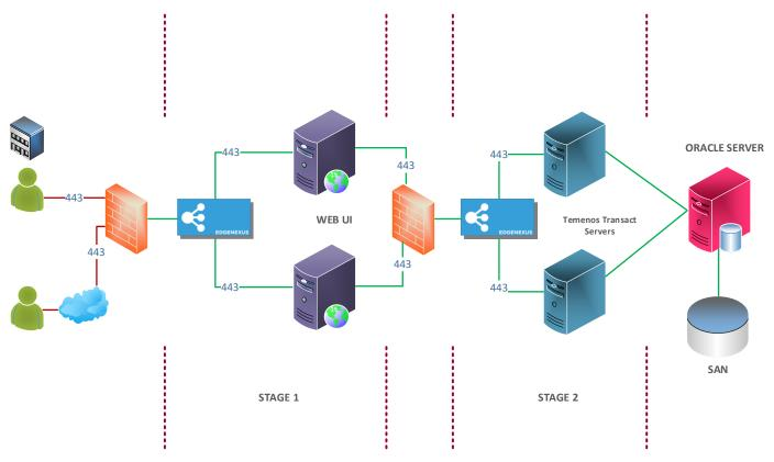
Stage 1 comprises the VIP and Virtual Services for load balancing the WebUI servers. These could be IIS, or as more sometimes used, Apache on Jboss.
